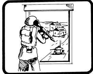
The gunner needs only the two meter safety distance from the rear bunker wall.
