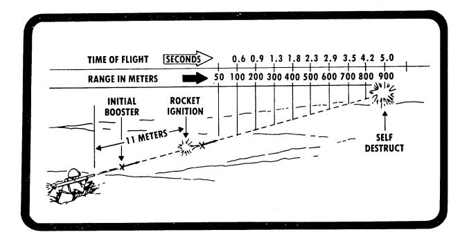
Note: The PG-7 grenade self-destructs approximately 900 meters from the launcher.
