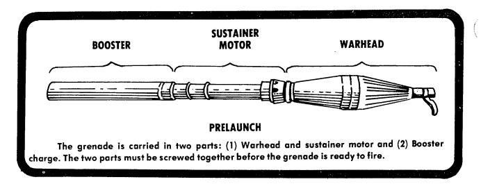
The PG-7 grenade is a rocket assisted projectile. It is first ejected from the launcher at a velocity of 117 meters per second by a small strip powder charge. This reduces backblast and protects the gunner. Approximately 11 meters from the launcher a sustainer rocket ignites and boosts the rocket to a maximum velocity of 294 meters per second. Thus the RPG-7 combines the advantages of reduced backblast with increased accuracy and range.
